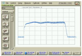
\*measured by 40GHz sampling oscilloscope with 20GHz optical channel
