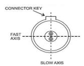
The output light is polarized along the slow axis of PM fiber.
