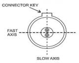
The output light is polarized along the slow axis of PM fiber.
